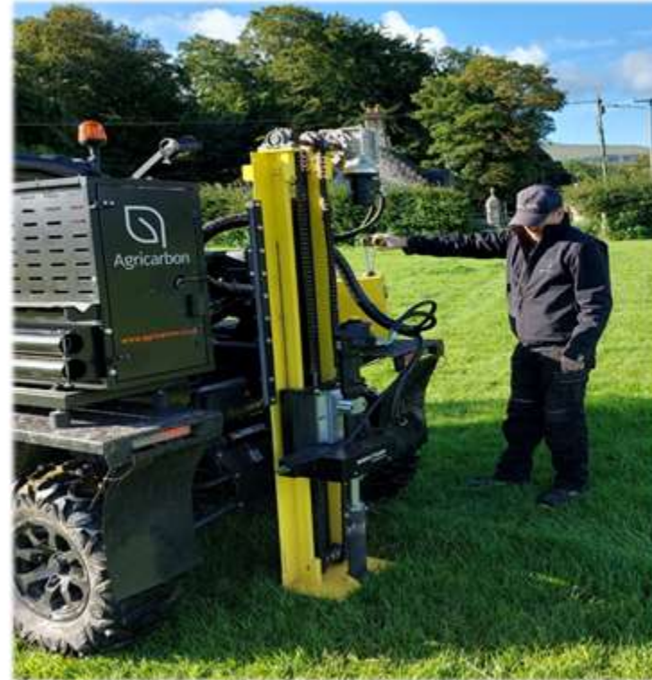
Soil Sampling to one metre deep
